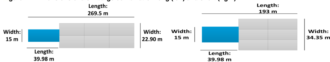
Figure 7.1 Dimensions of a six barge combination long (left) and short (right)
