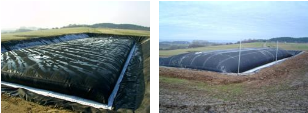
Figure 13: Examples for collapsible pillow fuel tanks made from rubber coated fabric [ (19)]
