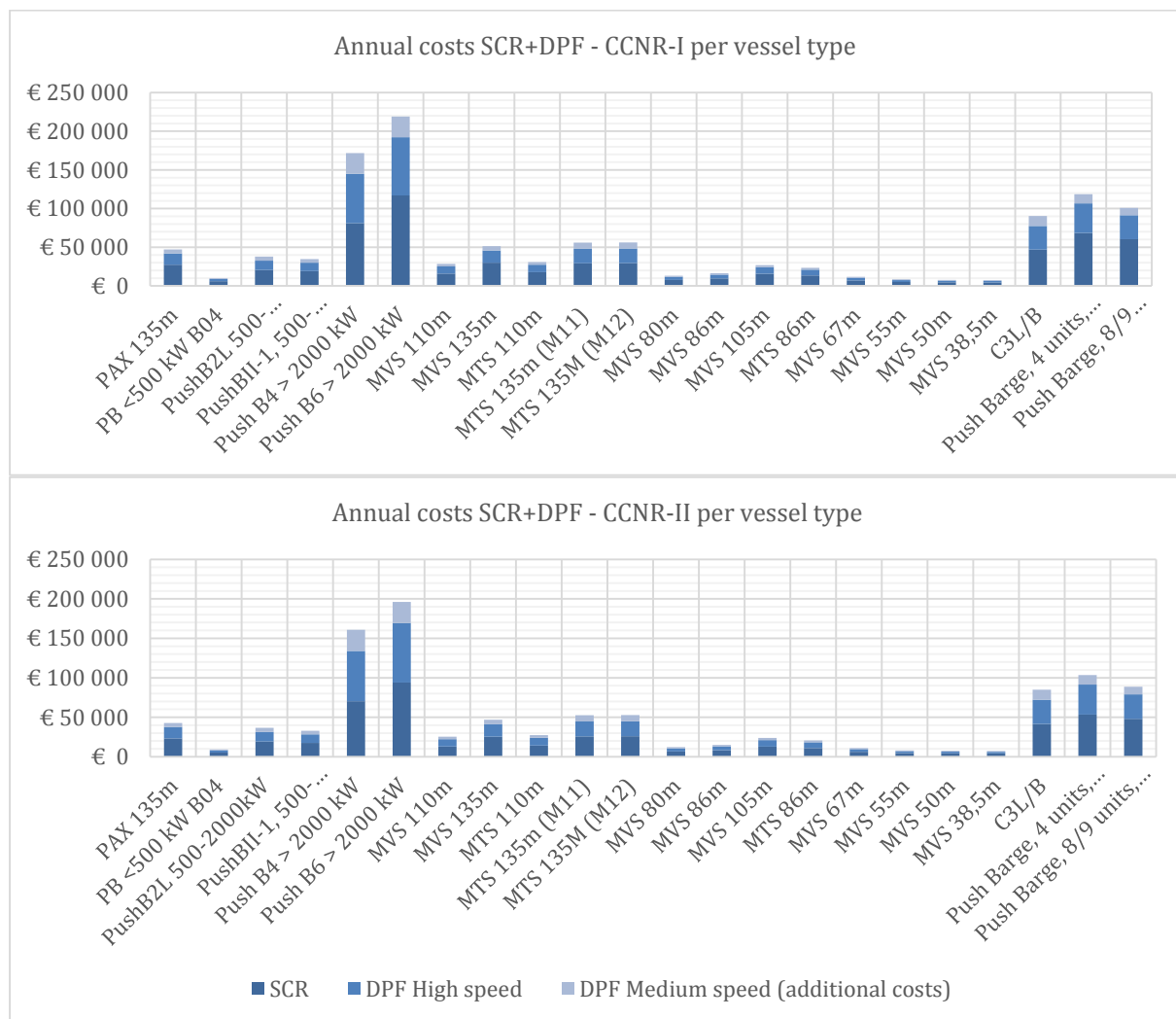
Figure 8: Annual costs SCR+DPF per vessel type for CCNR Stage-I and CCNR Stage-II engines (with the costs of SCR in dark blue, of DPF for high speed in medium blue and DPF for medium speed in light blue)
